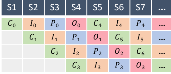
Figure 8: Cross-stacking view of CMU Groups. The S_i denotes the i -th MAU stage. The C_j , I_j , P_j , and O_j denote the four stages of CMU Group j listed in Table 2.
