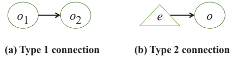
Fig. 2. Two types of connection in an ODG. (a) Type 1 connection: operation o_2 depends on the completion of operation o_1 . (b) Type 2 connection: event e can trigger operation o .
